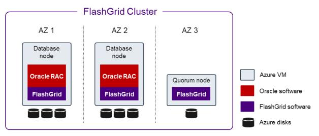
FlashGrid Cluster on Azure with two RAC database nodes
