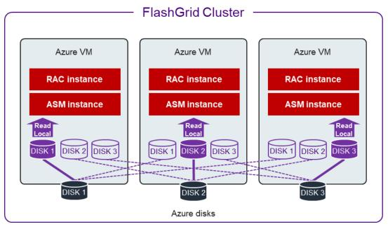
FlashGrid Storage Fabric software architecture on Azure
