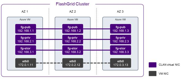
FlashGrid Cloud Area Network architecture on Azure
