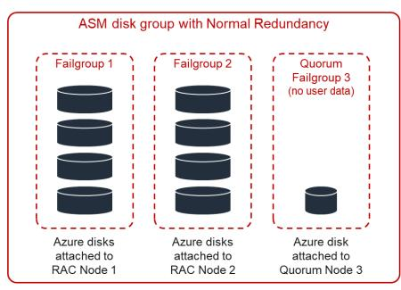
A Normal Redundancy disk group in a 2-node RAC cluster on Azure
