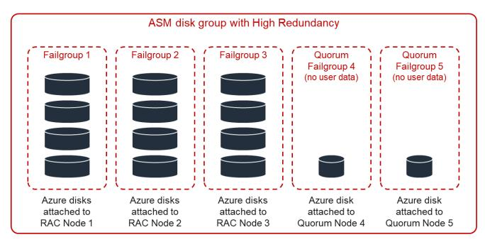
A High Redundancy disk group in a 3-node RAC cluster on Azure
