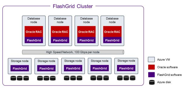
Extra-large database cluster on Azure with 4+ RAC nodes and separate storage nodes
