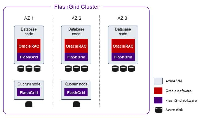
FlashGrid Cluster on Azure with three RAC database nodes
